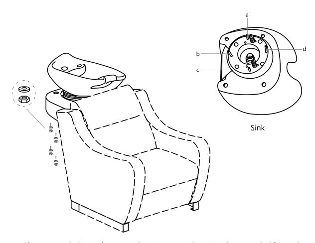
Undo the access panel by twisting clockwise then using the 4\* 14mm washers & gaskets provided fasten the sink to the base.
