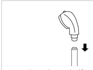
Unscrew the sprayerhead from the sprayer hose.
