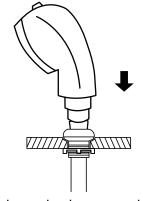
Place the sprayer hose from underneath throught the sprayerhead holder and fasten the sprayerhead to the sprayer hose.
