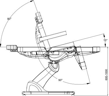
Dimension: 1780X880X600mm Minimum Height: 600mm Maximum Height: 1000mm N.W: 86kg Max load capacity: 180kg (normal use) Input voltage: AC 230V/50HZ Output Voltage: DC 24V
