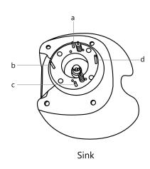
Undo the access panel by twisting clockwise then using the 4\* 14mm washers & gaskets provided fasten the sink to the base.
