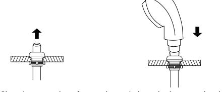
Place the sprayer hose from underneath throught the sprayerhead holder and fasten the sprayerhead to the sprayer hose.
