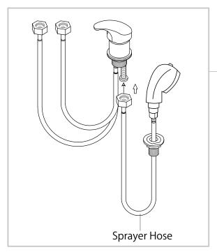
Connect to sprayer hose to the tap shown in the diagram.
