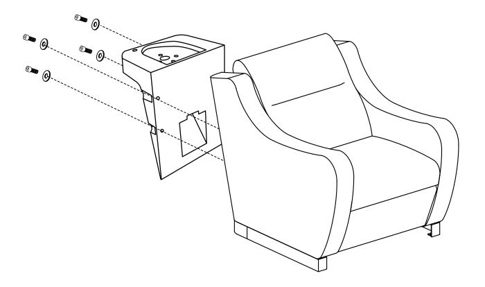
Secure the Cover on the back of the backwash.
