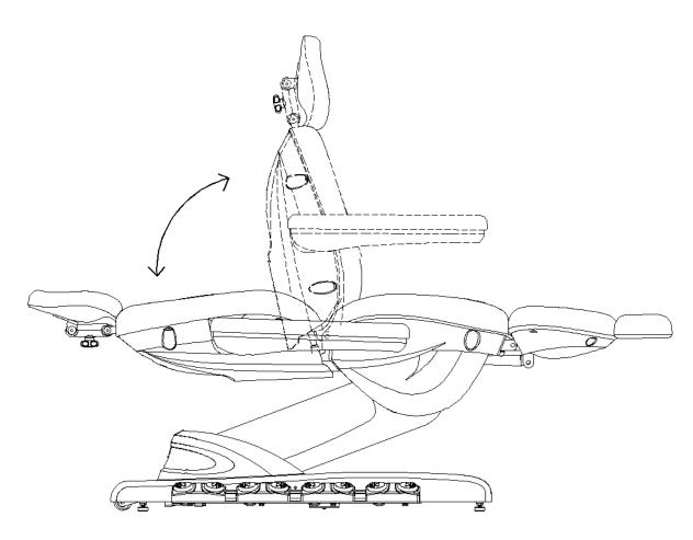
Step on A or B on the pedal control #2 to adjust the angel of the backrest, as shown in below picture
