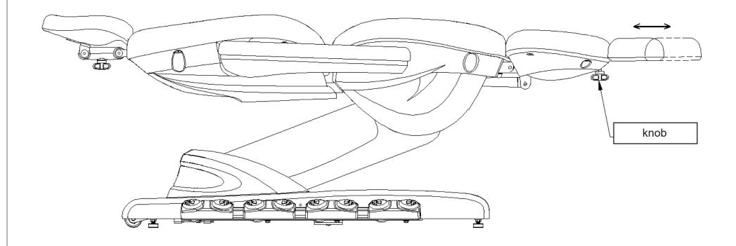
Adjust the extension of the footrest by loosening the knob under the footrest, as below picture shown.
