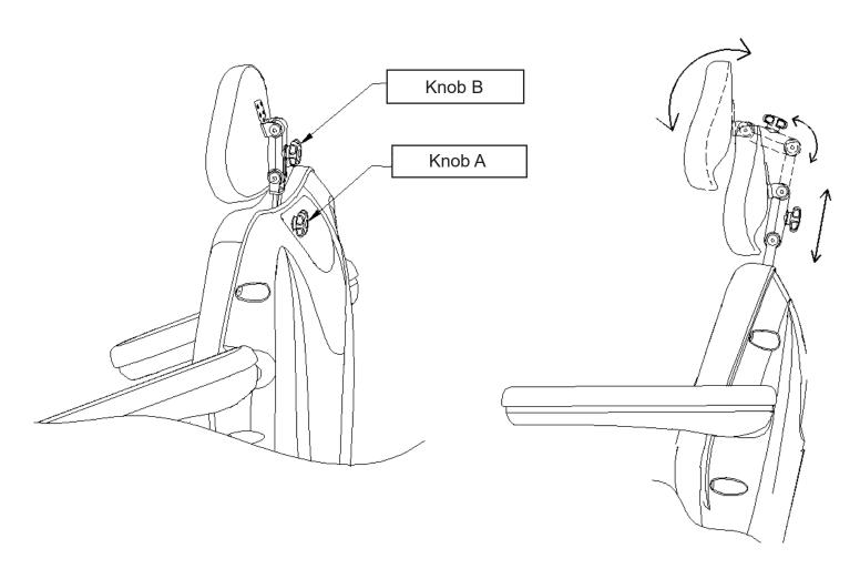
The height of the pillow can be adjusted by loosening knob A. You can rotate or flip over the pillow by loosen the knob B, as shown in below picture.
